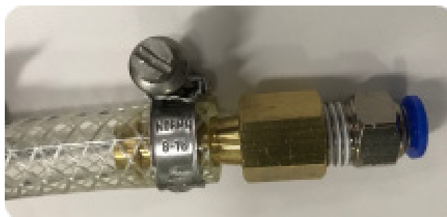
Attaching a Push-to-Connect Fitting to a Hose Barb Connector
